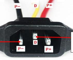
主板一线通接口黄色线接D SIF interface on the main board connects to D in yellow
