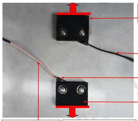
棕线为GSM天线 The brown one is a GSM antenna 注意: GSM天线与把手的"M"对应 Note: The GSM antenna corresponds to the "M" of the handle 注意: 钢片天线的横梁朝外安装 Note: The beam of the sheet steel antenna is mounted outwards
